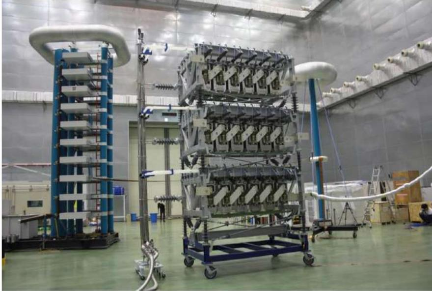
MMC: Modular Multilevel Converter
